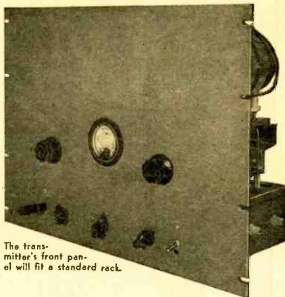
The transmitter's front panel will fit a standard rack.
