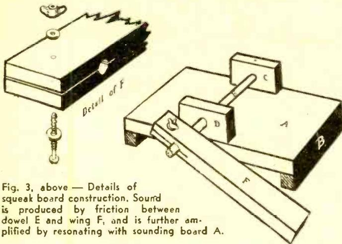
Fig. 3, above — Details of squeak board construction. Sound is produced by friction between dowel E and wing F, and is further amplified by resonating with sounding board A.
