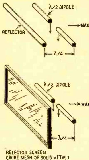
Fig. 1—The reflector may be a flat screen.
