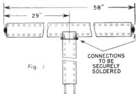
Fig. 1 shows how the antenna is made. The 300-ohm twin-lead transmission line may be type K-1046 (Federal Telephone and Radio) which is especially suitable because of its flexibility, weather-resistance, and very low loss. A 58-inch length of line is shorted at both ends after stripping the insulation as shown. The ends are twisted and soldered. Then one of the conductors
