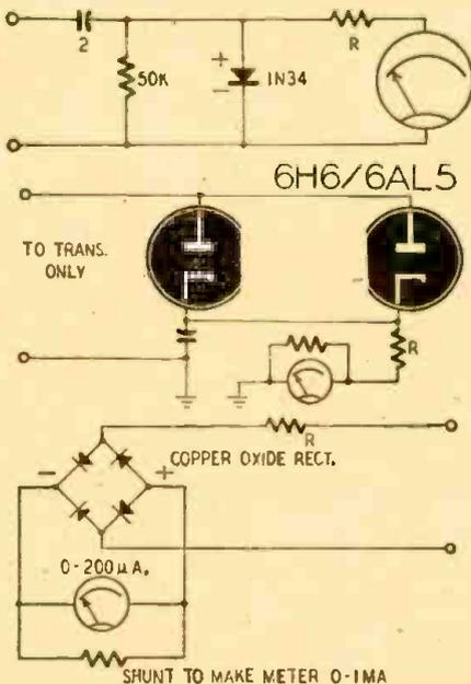
Fig. 3—Output meter rectifiers, three types.
