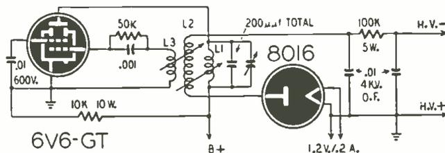
Circuit of the r.f. high voltage supply. Coil system is shown below.
