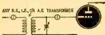
Fig. 4—A quick check method for r.f. coils.
