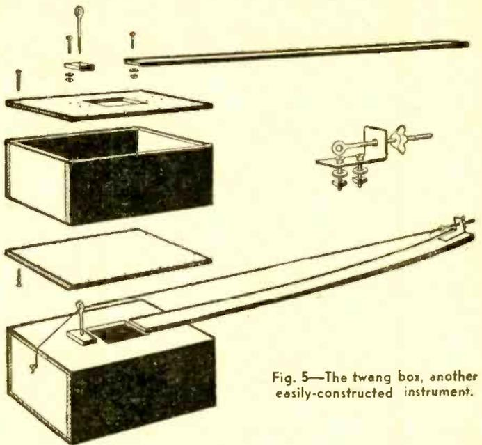
Fig. 5—The twang box, another easily-constructed instrument.
