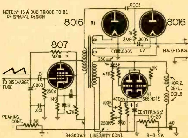
Fig. 6—An "inductive-kick" type of voltage-doubling power supply.
