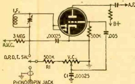
In some sets, the volume control is the entire detector load. In this instance, a 500,000-ohm resistor may be connected in the hot lead of the phono input circuit.
