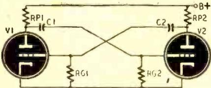
Fig. 1—The standard multivibrator circuit, consists of a 2-stage amplifier with the output of V2 fed back into the grid of V1. Due to the phase reversal of 180 degrees in each stage, the feedback voltage is in phase with the original impulse on V1 grid. Thus, the circuit satisfies the conditions necessary for oscillation—amplification with positive feedback.
