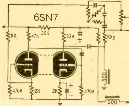
Good results will follow installation of Rx2 whether there is oscillation in the circuit or not. It should then be about 25,000 ohms.
