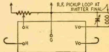
Fig. 10—Connections for modulation tests.
