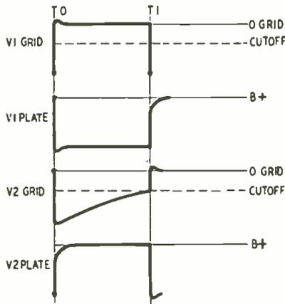
Fig. 6—Analysis of one-kick vibrator action.
